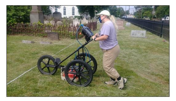
Plate 3. IUP Field Technician using GSSI SIR-4000 GPR system.
